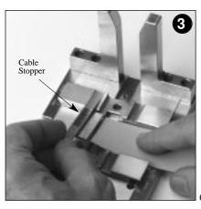
When installing a plug on the end of a cable, use the cable stopper to correctly position the cable.
