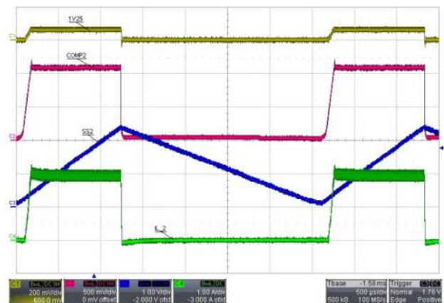
Figure 9: Synchronous Buck Hiccup Mode Operation when 1V25 is Shorted to GND and C_{SS2} = 10 nF
