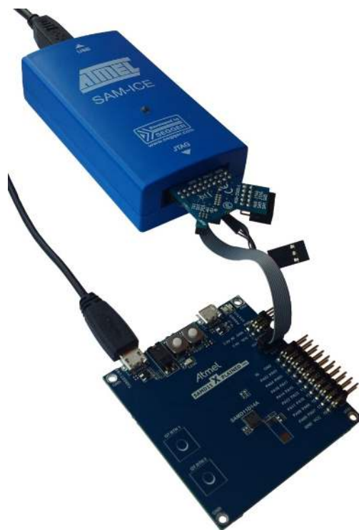
Figure 5-7. SAM-ICE using an Atmel-ICE Adapter
