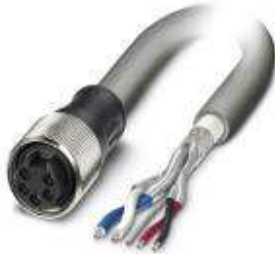
Bus system cable, DeviceNet, 5-position, PVC, Gray RAL 7001, Free cable end, on Socket straight 7/8"-16UNF, Cable length: 2 m
