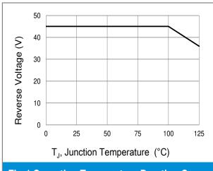
**Fig.4 Operating Temperature Derating Curve**
