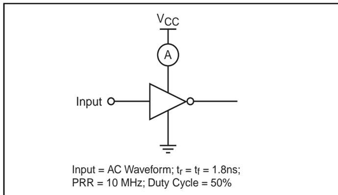
Figure 2. I<sub>CCD</sub> Test Circuit
