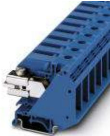
N disconnect terminal block, Special and hybrid connection, Cross section: 0.75 mm 2 - 35 mm 2 , AWG: 18 - 2, Width: 15 mm, Color: blue, Mounting type: NS 35/7,5, NS 35/15, NS 32
