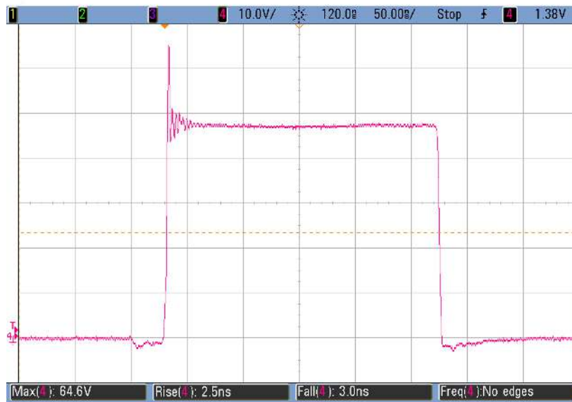
Figure 4: Typical waveforms for 48 V to 5 V / 20 A (400 kHz) CH4: switch node voltage
