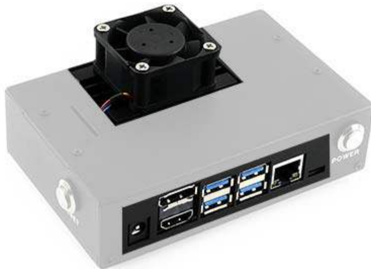
Opening for onboard connectors and cooling fan
