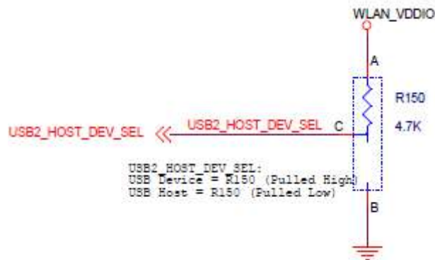
Figure 4-5. USB2_HOST_DEV_SEL Strapping Option
