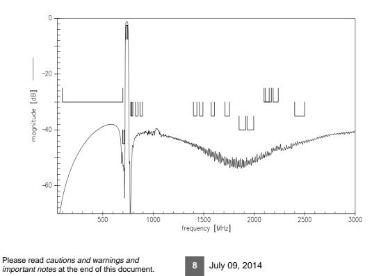
SAW ComponentsB8012SAW Duplexer707.5 / 737.5 MHz
