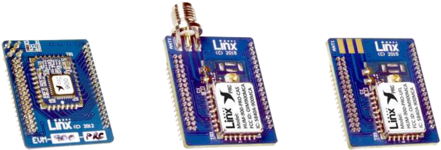
Figure 1: HumPRC™ Series Evaluation Modules; from left: EVM-***-PRC, EVM-***-PRC-CAS, EVM-***-PRC-UFL
