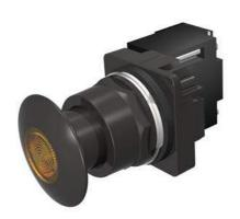
30mm BlackMax, Epoxy Coated Corrosion Resistant Complete Metal Unit Illuminated Push-Pull Operator Transformer type, 240V AC Incandescent Lamp Mushroom Head Cap Small 1 3/4" (44.5 mm) Metal, Black with Amber Lens 3 Position Pull-Momentary/Push-Maintained UL Listed, CSA Certified NEMA 1,3,3R,4,4X,12,13 & Automotive Standards
