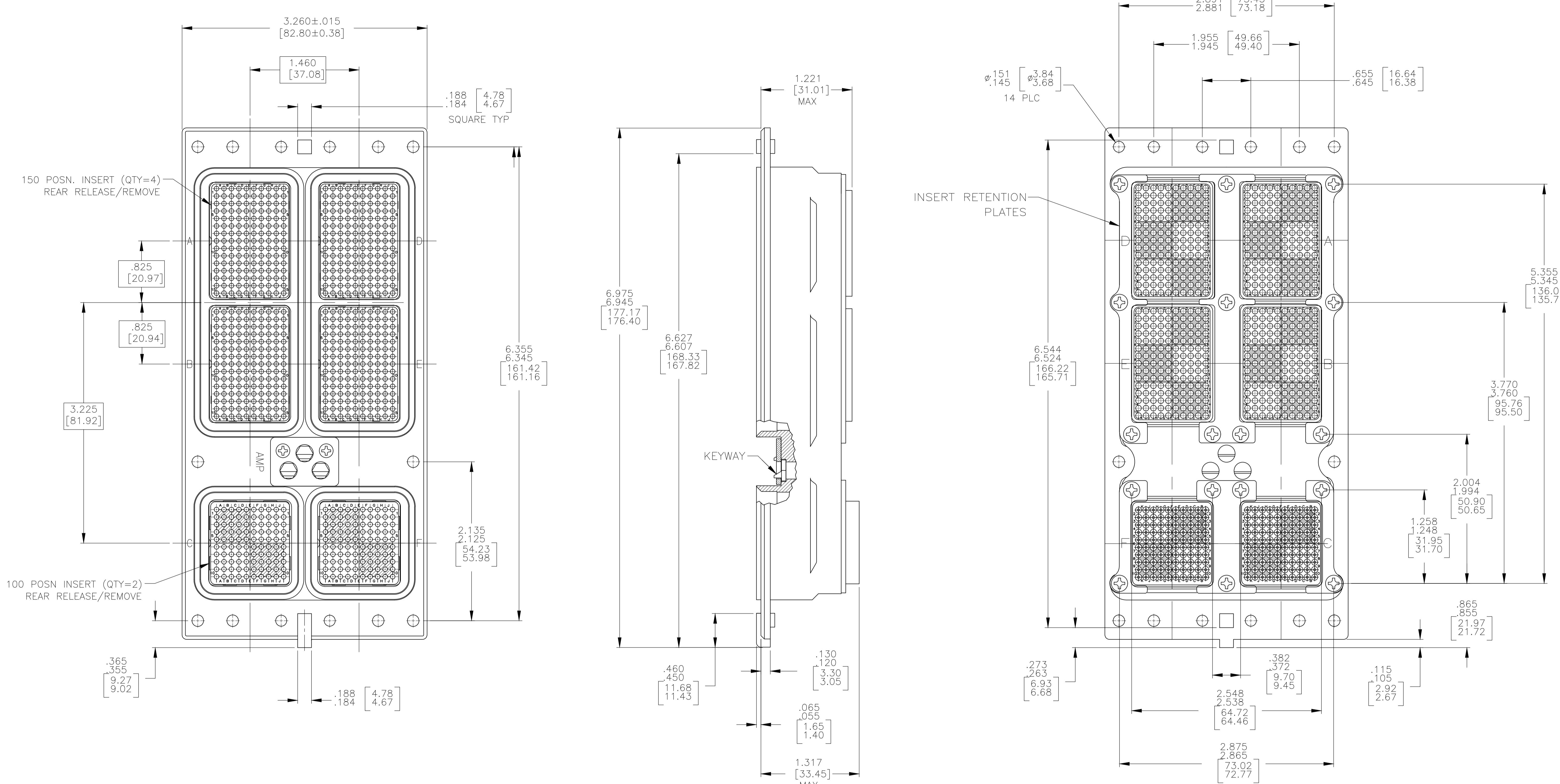
1. CONNECTOR DIMENSIONS ARE PER ARINC 600 SPECIFICATION
