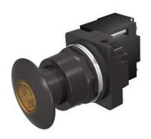
30mm BlackMax, Epoxy Coated Corrosion Resistant Complete Metal Unit Illuminated Push-Pull Operator Transformer type, 480V AC Incandescent Lamp Mushroom Head Cap Small 1 3/4" (44.5 mm) Metal, Black with Amber Lens 2 Position Maintained, Pull-to-Release UL Listed, CSA Certified NEMA 1,3,3R,4,4X,12,13 & Automotive Standards
