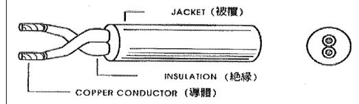
Conductor construction: 26/0.254±0.008 Insulation outer diameter:Ø3.05±0.1 Insulation Thickness:Minimum 0.69 mm: Coated outer diameter:Ø7.8 ± 0.2 Coating Thickness:Minimum 0.61mm
