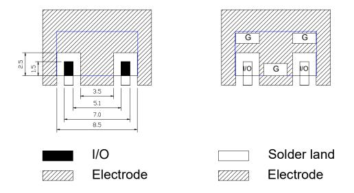
Shielding case layout guide (MIN)
