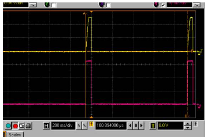
FIGURE 14. DYNAMIC CURRENT LOOP STARTED TO ENABLE. TOP IS VLNb AND BOTTOM IS LOAD CURRENT WAVEFORM (200mA/DIV)
