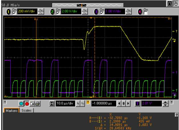
FIGURE 21. ENT BIT GOING HIGH TO TONE ENABLED ON THE OUTPUT DELAY IS ~34μs
