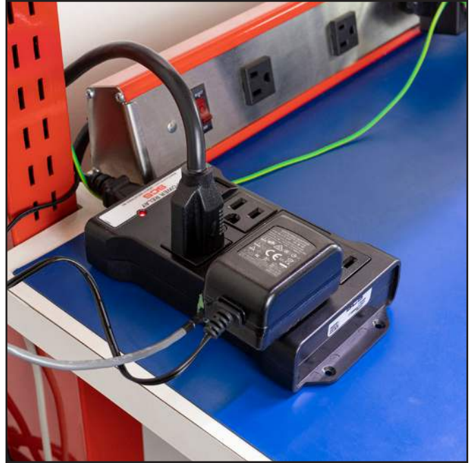
Figure 10. Using the SCS 770069 Power Relay to power a workbench and the WS Aware Monitor
