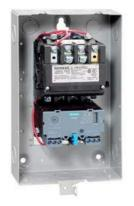
Non-reversing motor starter Size 1 Three phase full voltage Solid-state overload relay OLRelay amp range 0.25-1A 190-220/220-240V 50/60HZ coil Combination type Indoor general purpose use
