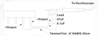
A 30cm twisted pair of no.18 AWG copper wire is connected to a 47uF and 0.1uF capacitor of proper polarity and voltage rating. The oscilloscope probe ground led should connect right to the ground ring of the probe and be as short as possible. The oscilloscope bandwidth should be at 20MHz and connected to AC ground.
