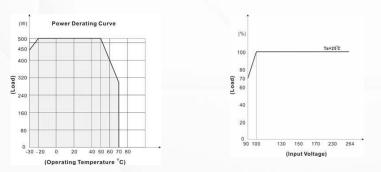
If input voltage is lower than 100VAC, please refer to the output derating V.S. input voltage curve for details
