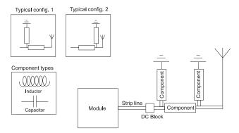
The matching network has to be individually designed using one, two or three components.
