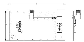
The testboard is designed for evaluation purposes for the Flavus 2.4 GHz antenna. The card has the same size as a typical PCMCIA card and is fitted with an SMA connector.
