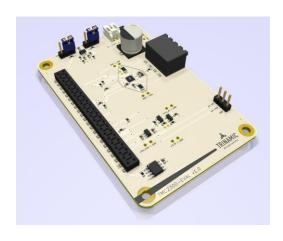
The TMC2300-EVAL is part of TRINAMICs universal evaluation board system which provides a convenient handling of the hardware as well as a userfriendly software tool for evaluation. The TMC2300 evaluation board system consists of three parts: Landungsbrücke (base board), Eselsbrücke (connector board with test points), and TMC2300-EVAL.
