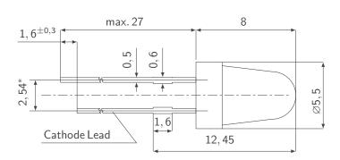
all dimensions in mm. Tolerance  $\pm 0,\, 1$  except given ones \* at the bottom of the LED
