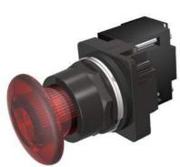
30mm BlackMax, Epoxy Coated Corrosion Resistant Complete Metal Unit Illuminated Push-Pull Operator Transformer type, 600V AC LED Lamp Mushroom Head Cap Small 1 3/4" (44.5 mm) Plastic, Red 3 Position Pull-Momentary/Push-Maintained UL Listed, CSA Certified NEMA 1,3,3R,4,4X,12,13 & Automotive Standards
