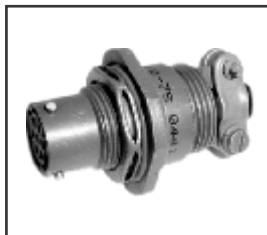
62 IN - 14F Single hole mounting with grommet and grommet nut fitted with integral strain relief clamp has panel 'O' ring seal
