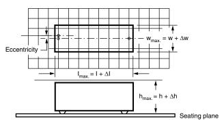
For the minimum product dimensions for length ( $l_{min.}$ ), width ( $w_{min.}$ ), and height ( $h_{min.}$ ) following tolerances of the components are valid:
