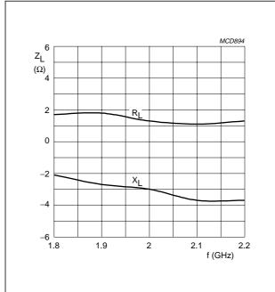
$V_{DS}$  = 26 V;  $I_{DQ}$  = 180 mA;  $P_L$  = 45 W;  $T_h \leq$  25 °C.
