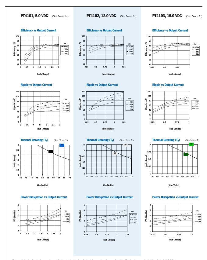
Note A: All data listed in the above graphs, except for derating data, has been developed from actual products tested at 25°C. This data is considered typical data for the DC-DC Converter.
