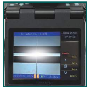
Fusion splicing finish
