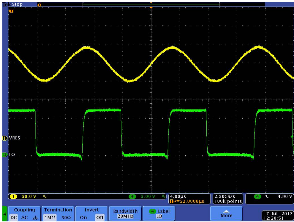
Figure 12. Voltage on Resonant Capacitor ( V_{in} = 390\text{-V} and 10-A Load, Ch1 = V_{RES} ; Ch4 = LO)
