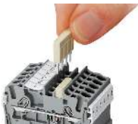
Insert push-in type jumper bar and push down until it hits backstop.
