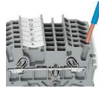
Inserting a conductor via push-in termination: Solid conductors with cross-sections from either one size above, or up to two sizes below, the rated cross-section can be simply pushed in – no tools needed.
