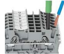
Inserting a conductor via operating tool: Connecting fine-stranded conductors without ferrules, or small cross-sectional conductors that cannot be pushed in, is performed similarly to the original CAGE CLAMP® – just use an operating tool. Advantage: To open the clamp, the operating tool is inserted vertically. The conductor entry is less than 15 degrees for easier wiring.
