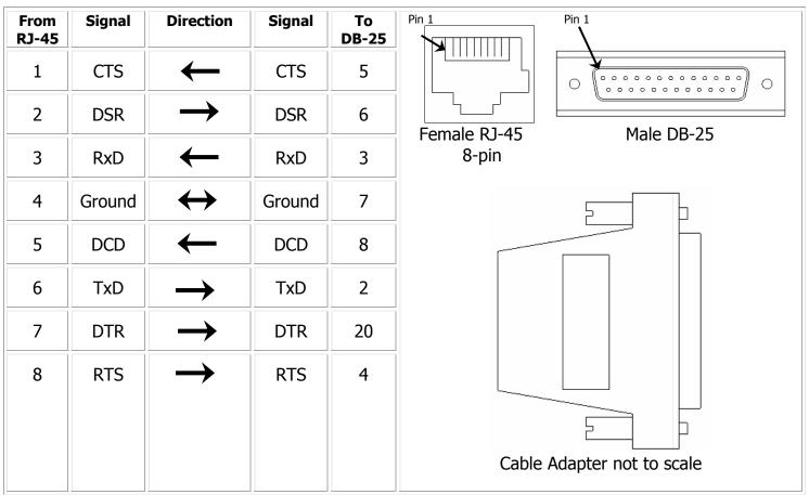
\* Arrows indicate which direction the signal is flowing
