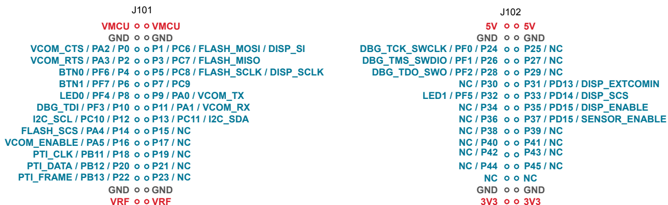
Figure 4.2. Radio Board Pin Mapping on Breakout Pads
