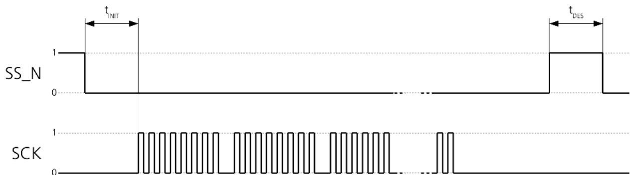
Figure 3: SPI timing diagram
