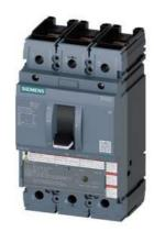
circuit breaker 3VA5 UL frame 250 breaking capacity class C 100kA @ 480 V 3-pole, line protection TM210, FTFM, In=250A overload protection Ir=250A fixed short-circuit protection Ii=10 x In UL489 SB (naval), 50 deg. cel. nut keeper kit on both sides
