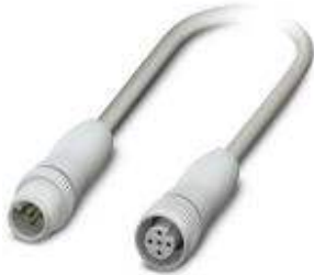
Sensor/Actuator cable, 5-position, PP-EPDM halogen-free, Gray RAL 7035, Plug straight M12, A-coded, on Socket straight M12, A-coded, Cable length: 1.5 m, Hygienic design, with plastic knurl
