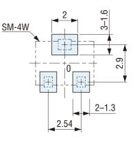
Note) The zero point is the center of mounting.
