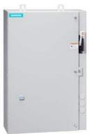
Reversing motor starter, Size 3, Three phase full voltage, Solid-state overload relay, OLR amp range 25-100A, 110V 50Hz / 120V 60Hz coil, Combination type, 100A disconnect switch, Enclosure NEMA type 4/12, Water/dust tight for outdoors
