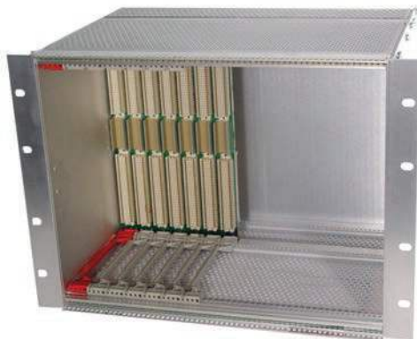
CCA28-64-01 with perforated top/bottom covers and Vector 7-slot VME64x backplane
