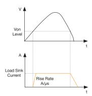
Control the input turn on state for the DC electronic load by configuring the Von latch functions. This can be used to start and stop discharging of a battery or other power source once a specified voltage level is reached.
