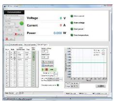
PC software is provided for front panel emulation, generating and executing test sequences, or logging measurement data without the need to write source code. Additionally, this application software integrates with NI Data Dashboard for LabVIEW applications, allowing users to create a custom dashboard on a tablet computer or smart phone to remotely monitor 8500B Series DC loads.
