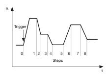
List mode lets you generate more complex sequences of input changes with several different levels. Save up to 7 groups of list files to internal memory for recall and set parameters including step counts (range 2 to 84), width time of a single step (minimum 20  $\mu s$ ), step value, and slope.
