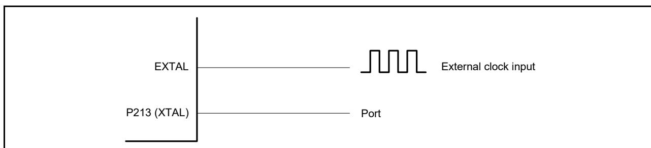
Figure 9.8 Equivalent circuit for external clock
