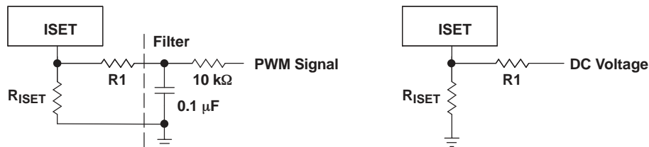
Figure 19. Analog Dimming Uses an External Voltage Source to Control the Output Current
