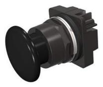
30mm BlackMax, Epoxy Coated Corrosion Resistant Metal Operator, Round Push-Pull Operator Non-Illuminated Mushroom Head Cap Small 1 3/4" (44.5 mm) Plastic, Black 3 Position Pull-Momentary/Push-Maintained UL Listed, CSA Certified NEMA 1,3,3R,4,4X,12,13 & Automotive Standards
