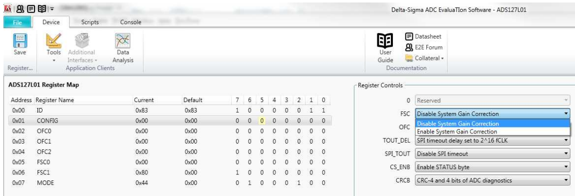
Figure 6. Register Controls for the ADS127L01
