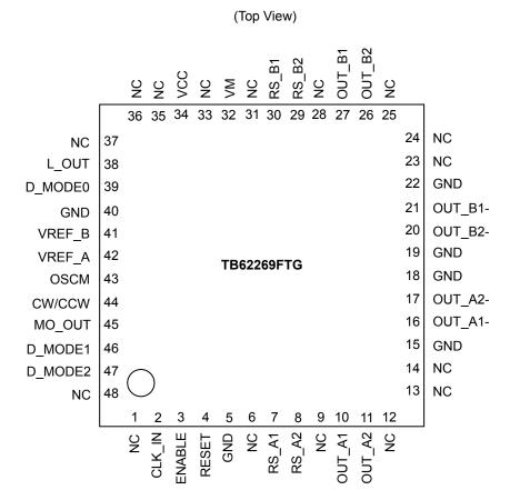
X Please mount the four corner pins of the QFN package and the exposed pad to the GND area of the PCB.
