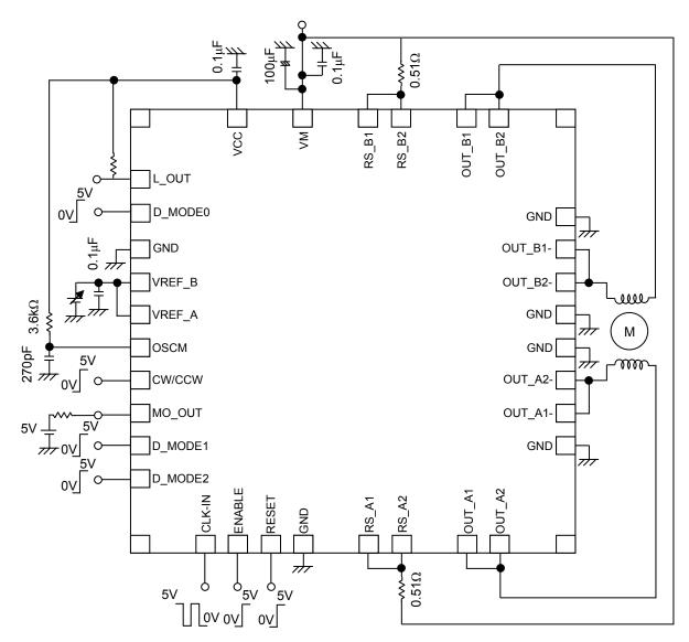
Note: I will recommend the addition of a capacitor if necessary. The GND wiring must become one point as much as possible-earth.
