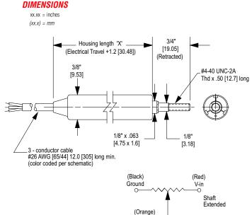
Caution: Do not test on an Ohm Meter on the Rx 1 scale or other current devices. Caution: Excessive Wiper Current can cause Output errors or damage. Caution: Zero shaft side load is recommended to achieve maximum life.
