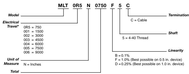
Note: Not all combinations are available. Minimum quantity orders apply. Contact the factory for more details. \* Note: The *Electrical Travel* correlates to the *Total Resistance (Ohms)*.
