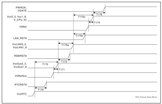
Figure 16-19. 1.8 V/3.3 V Power Sequencing
