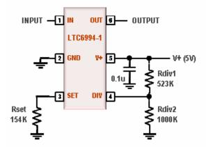
DC1562A-L, 100MS DELAYED OUTPUT EDGE FROM INPUT EDGE, BOTH RISING AND FALLING EDGES
