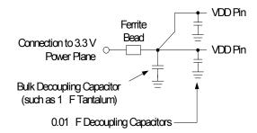
Both VDD pins must be connected to the same voltage.
